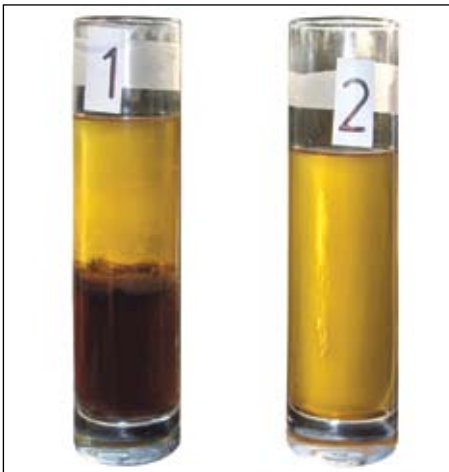
Contaminated (1) and polished (2) fuel.
